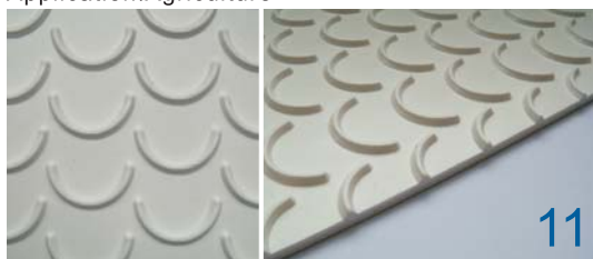
Name:Crescent Thickness:2.2mm Property:Incline conveying Application:Poultry, Sea food processing
