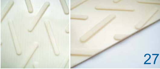
Name:Staggered stud Thickness:1.8mm Property:Incline conveying,easy clean Application:Tobacco
